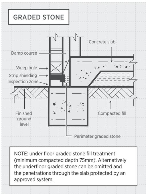
NOTE: under floor graded stone fill treatment (minimum compacted depth 75mm). Alternatively the underfloor graded stone can be omitted and the penetrations through the slab protected by an approved system.
